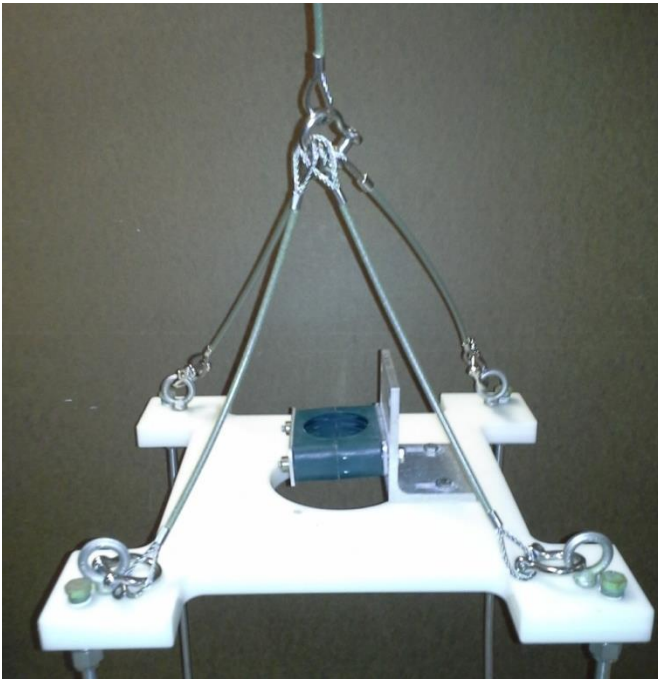
Figure 77 - All metal lanyards and shackles are attached
