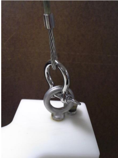
Figure 75 - Example of shackle and metal lanyard attached to eyebolt
