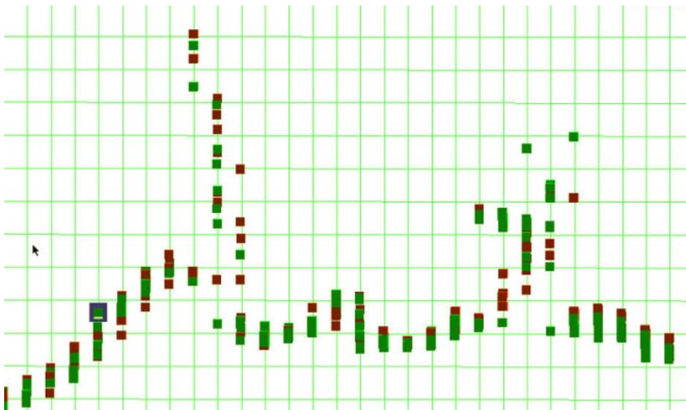
Figure 12. Soundings from two separate lines crossing LCT 524. Color represents the individual lines. Note the consistency of position of the soundings on the gunnels from line to line. Grid cells represent 50 cm distance.
