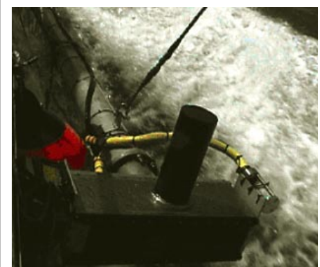
Figure 4b. Reson 8125 and sound speed sensor mounted on pole (in non-deployed position).
